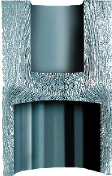
Consistent grain flow results in a stronger socket. Material stays in the walls through precisely milled raw stock and cold forging.
